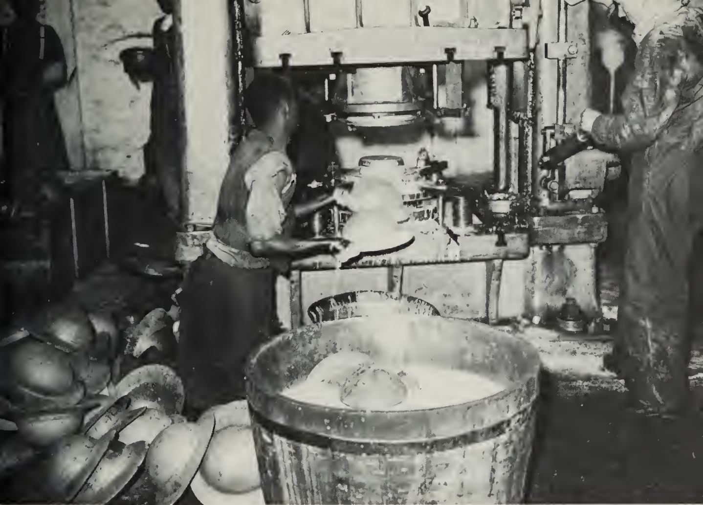
Pressing steel helmets for Springbok troops. A young iron and steel industry at Pretoria is the backbone of the Union's arms and munitions production.
